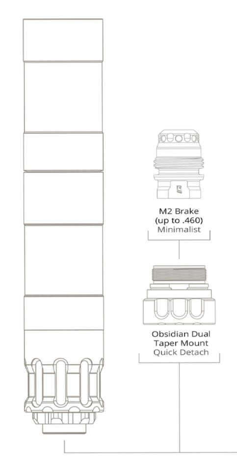
\*The M2 Brake has thread pitch options that are compatible with projectiles up to a .460 diameter. Make sure that the suppressor being used is also compatible with that caliber. For instance, the M2 Brake in 5/8x24 can be used with 45-70 for the Obsidian45, but not the Obsidian9.
