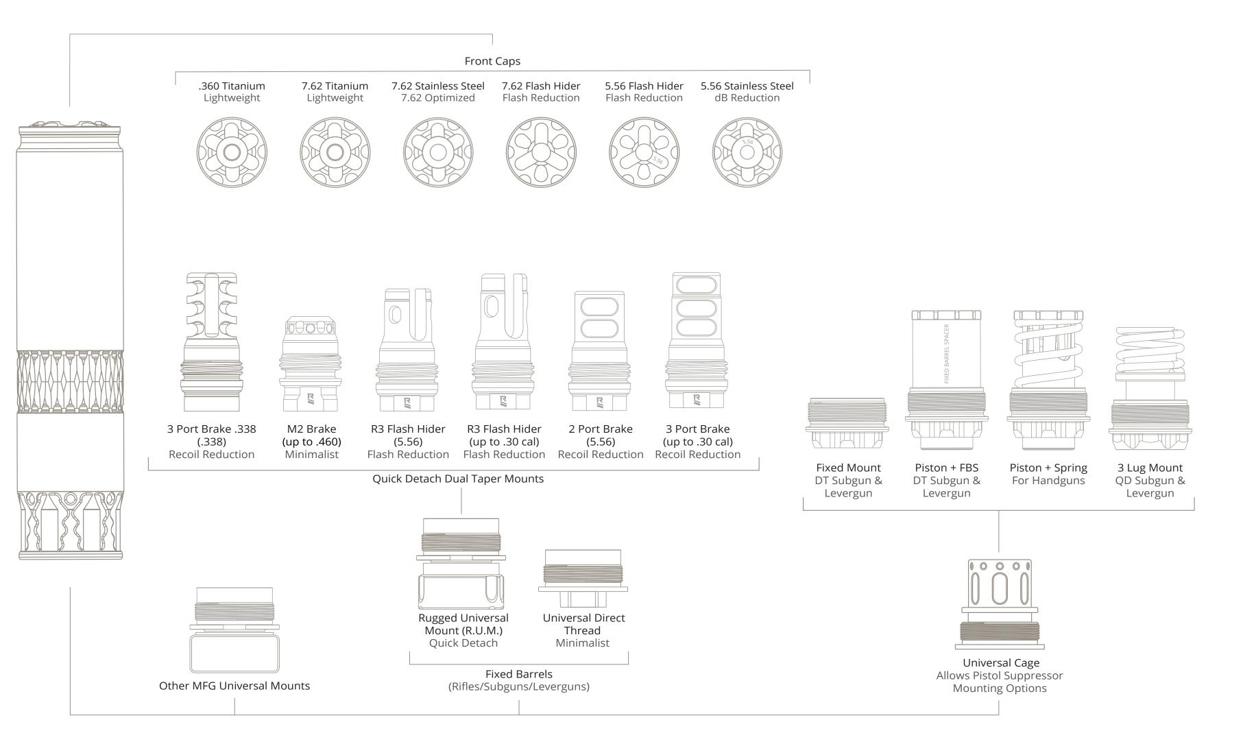
\*The M2 Brake has thread pitch options that are compatible with projectiles up to a .460 diameter. Make sure that the suppressor being used is also compatible with that caliber. For instance, the M2 Brake in 5/8x24 can be used with 45-70 for the Obsidian45, but not the Alaskan series.
